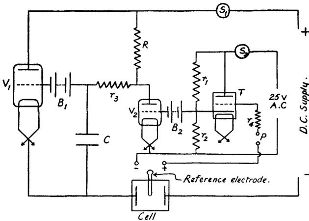
FIG. 1.—Potentiostat Circuit.
