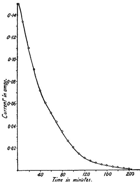
FIG. 5.—Electrolysis of copper sulphate solution at constant potential.
