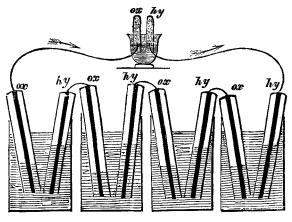
axis of the tube platinized platina foil, which in the battery I constructed was about one-fourth of an inch wide. It is obvious that, by allowing the platina to touch the liquid, the latter would spread over its surface by capillary action and expose an extended superficies to the gaseous atmosphere. The battery was charged with dilute sulphuric acid, sp. gr. 1.2, and the following effects were produced:—
